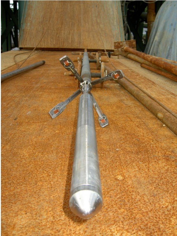
DIP – slimhole wireline Dipmeter tool
