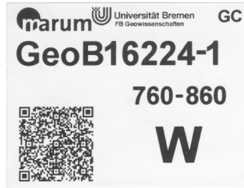
Fig. 5.8: IGSN encrypted in QR code on core sample
