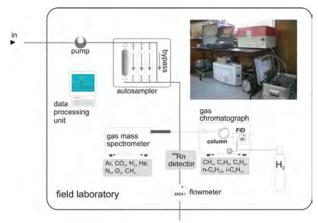
Fig. 5.12: Flow path of gas analyses steps
