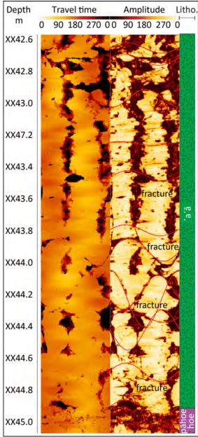
Fig. 4.6.12: Fractures on an acoustic image log
