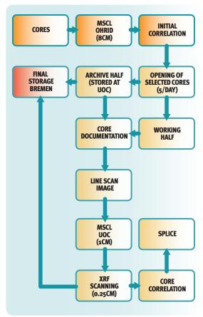
Fig. 4.5.10: Core handling workflow during the Lake Ohrid drilling expedition.
