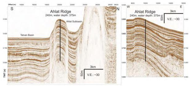
Fig. 4.1.13: Crossing high-resolution seismic profiles at a suggested drill sites in Lake Van, Turkey, in which only a combined interpretation of both profiles allows understanding the structural context of the suggested site, modified after Litt et al. (2009) and Cukur et al. (2014)
