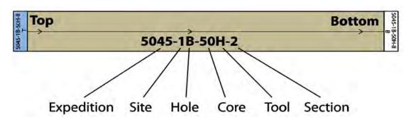
Fig. 4.5.8: ICDP standard core labelling routine. Arrows point to the bottom of the core, blue caps are attached to the top, white caps to the bottom of each core section.
