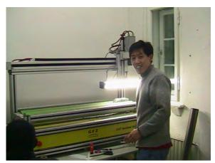
Fig. 5.10: Optical core scanner in operation
