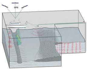
Fig. 4.1.7: Potential setup for an acoustic lacustrine site-survey with multibeam bathymetry (left) sediment echo sounder (center), reflection seismic system (right)
