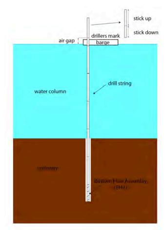
Fig. 4.5.9: Simplified scheme for the illustration of the drill depth calculations
