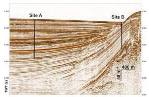
Fig. 4.1.14: Drilling at site A allows to recover a complete section of undisturbed sediments. Instead of deepening site A, older sediments can be drilled at site B at much lesser drilling depth. Modified after Wagner et al. (2014).
