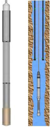
Fig. 4.6.2: Sketch of a sonde combination comprising total gamma ray, spectrum gamma ray and magnetic susceptibility, from top to bottom (left). A logging sonde is run through a coring drill string and the bit after the inner core barrel has been pulled out (right).
