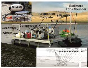
Fig. 4.1.10: Setup of an airgun reflection seismic system consisting of a Micro-GI Gun (modified Mini-GI Gun), a single mobile diving compressor, an air bottle for intermediate storage of compressed air, a 50-long 32 channel digital streamer and an acquisition system; upper left: image of a Mini-GI gun; lower right: principle of seismic reflection profiling.
