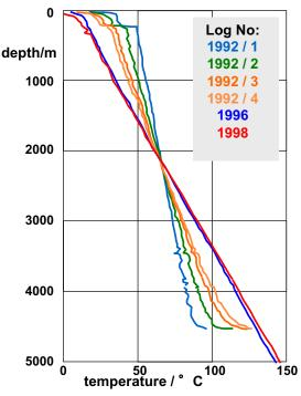
Fig. 4.6.6: An example of temperature equilibration in a deep borehole. The curves from 1992 were measured after the hole was drilled to 4500 m.
