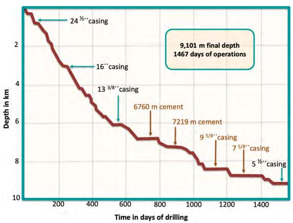
Fig. 3.4.1 Depth versus duration of drilling for the KTB well in Germany. Note that duration and costs are directly correlated. Major delays marked with brown arrows caused major cost increases.
