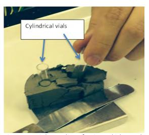
Fig. 4.5.11: Sub-sampling of a 2 cm-thick sample slide using cylindrical vials. The latter collect predefined volume samples parallel to the long axis of the core in a top to bottom direction, which enables the calculation of the water content, and thus dry and wet bulk density, respectively.
