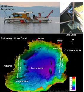
Fig 4.1.8: Upper left: Multibeam transducer mounted at the bow of a small survey vessel. Upper right: Details of the multibeam transducer. Lower part: Bathymetric map of Lake Ohrid collected with a multibeam system (taken from Lindhorst et al., 2012)
