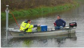
Fig. 4.1.9: Shallow water survey with parametric sub-bottom profiler SES-2000 consisting of a transducer and a control unit and consuming less than 500 W (© Innomar Technologie GmbH 2006)
