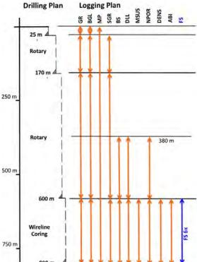
Fig. 4.6.4: Example of an optimized logging plan. GR: total gamma ray, BGL: borehole geometry, MP: mud parameter, SGR: spectrum gamma ray, BS: sonic, MSUS: magnetic susceptibility, NPOR: neutron porosity, DENS: density, ABI: acoustic imager, FS: fluid sampler
