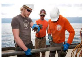
Fig. 4.5.7: Drill core handling on the barge. Small holes were drilled into plastic liners to prevent excessive core expansion from high gas pressure in the liner (Photo: N. Leicher).
