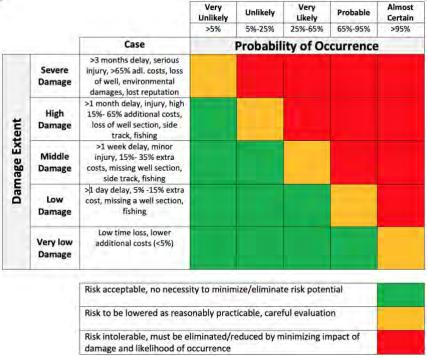
Table 3.7.2: Damage Extent vs Probability matrix for drilling projects
