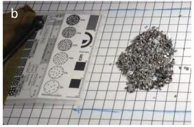
Fig. 4.5.19: Photographs of a) NanTroSEIZE cuttings (> 4 mm) separated in sandstone, silty claystone, fine silty claystone, and cement (from casing). The label in the upper part shows the expedition, drill site, drill hole, material number, method (solid taken from mud water), and the working portion; b) DFDP cuttings (all grain sizes) with percentage of area, sorting, roundness etc. for later description.
