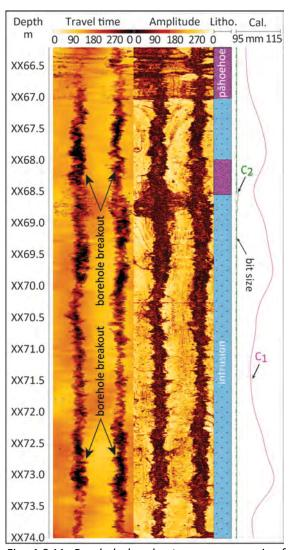
Fig. 4.6.11: Borehole breakouts appear as pair of dark, patchy stripes on opposing sides of the wellbore wall characterized by low amplitude and high travel time values.
