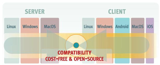
Fig. 4.3.7: The main mDIS (server) will be installed on a virtual box, which can run on Linux, Windows and MacOS. As long as a device has a web browser it can access mDIS.
