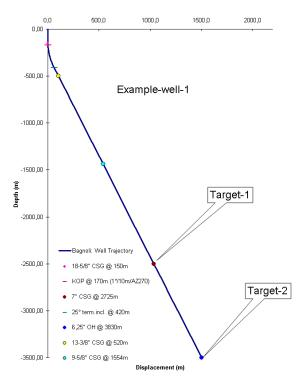
Fig. 4.2.10: Directional well plan for Campi Flegrei project in Italy
