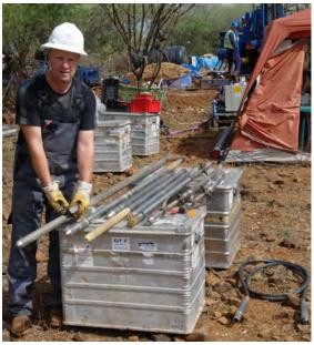
Fig. 4.6.15: OSG slimhole wireline logging sondes at a drill site
