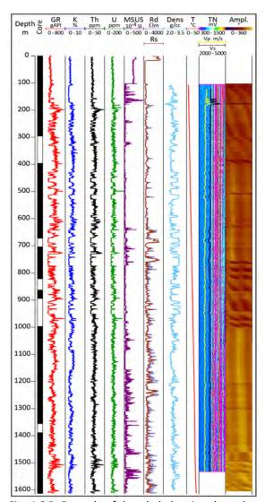
Fig. 4.6.5: Example of downhole logging data plot. Core recovery (left column; black = core recovery) and a compilation of downhole logs (from left: total natural gamma ray, contents of U, Th, K, magnetic susceptibility, resistivities (Rd and Rs; deep and shallow resistivity, respectively), density, temperature, sonic and amplitude borehole wall image).
