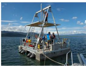
Fig. 4.1.12: Platform for taking shallow piston cores
