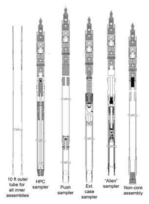
Fig. 4.2.5: Tools used for coring lake sediments
