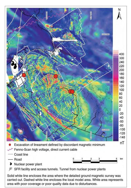
Fig. 4.1.6: Integrated total magnetic field from Forsmark, Sweden, based on data from a helicopter airborne survey in a N-S direction and a high-resolution ground magnetic survey in a NNW-SSE direction. Units in nanoTesla [nT]. Locations of investigations of lineaments defined by magnetic minima are also shown. Figure is from Stephens et al. (2015).
