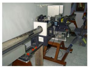
Fig. 5.9: Multisensor core logger in field lab
