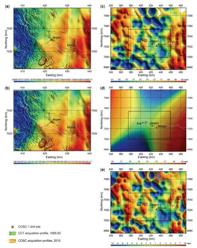
Fig. 4.1.2: (a) Observed total field aeromagnetic anomaly; (b) residual magnetic field after removal of the magnetic reference field (DGRF); (c) observed Bouguer gravity anomaly; (d) regional gravity field; and (e) Bouguer-residual gravity field. The black rectangle shows the extent of data used in the inversion modeling of Hedin et al. (2014).
