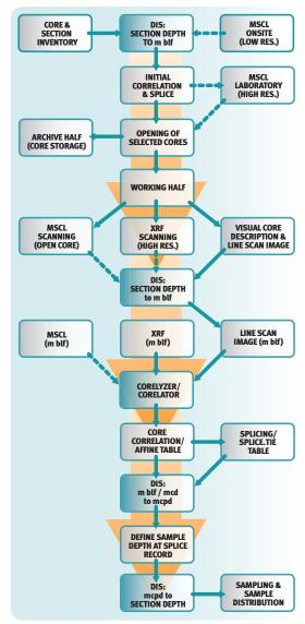
Fig. 4.5.13: Schematic workflow for the laboratory work and data management for lake drilling projects (mblf: meters below lake floor, mcd: meters corrected depth, mcpd: meters composite depth). The workflow is adopted using the workflow applied for Lake Ohrid data using the old DIS data management tool. The new workflow is work in progress.
