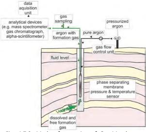
Fig. 4.7.9: Mode of operation of Gas-Membrane Sensor (GMS) and experimental workflow
