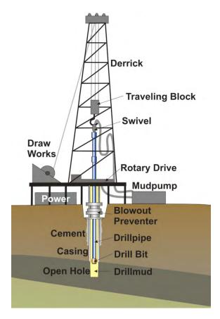
Fig. 4.2.1: Key components of rotary drilling
