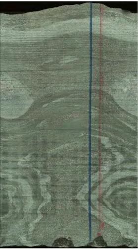
Fig. 4.5.3: Whole round optical core scan of gneiss core section showing double reference line in upright position with red line on the right
