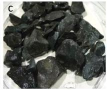
Fig. 4.5.17(a) cuttings of mica schist taken during the DFDP drilling project in New Zealand, (b), cuttings of a mixture of sand/silt and claystone taken from the SAFOD drilling project in USA, (c) cuttings of silty claystone, siltstone and sandstone taken during the NanTroSEIZE drilling project in Japan (cm scale).
