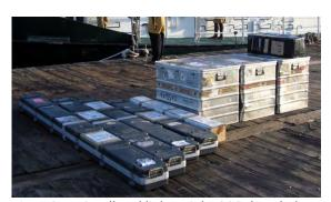
Fig. 4.6.14: Small and lightweight OSG downhole logging equipment ready to be shipped.
