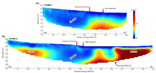
Fig. 4.1.5: ERT results along two profiles from central Sweden consistently showing clear evidence of a conductivity structure west of a scarp. The data also suggest that the bedrock is shallower on the eastern side of the scarp than on its western side, consistent with magnetic and seismic results. Figure is from Malehmir et al. (2016).
