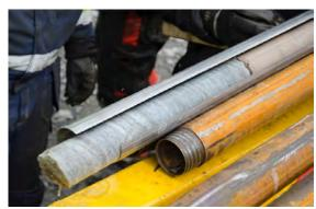
Fig. 4.5.1: First COSC drill core (gneiss below cement) in opened inner tube of a triple tube core barrel assembly. Clearly visible is the split aluminium liner protecting core from external forces, the second tube, and the drill string tube, hence 'triple tube'.
