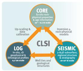
Fig. 4.6.8: The CLSI method integrates and connects several investigation methods at different scales
