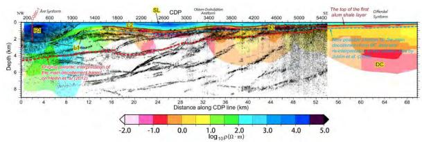
Fig. 4.1.4: 2D resistivity model from Yan et al. (2017). The depth to the good conductor east of CDP 1500 corresponds very well to the top of the strong reflectivity in the seismic section. For details on interpretation see Yan et al. (2017).
