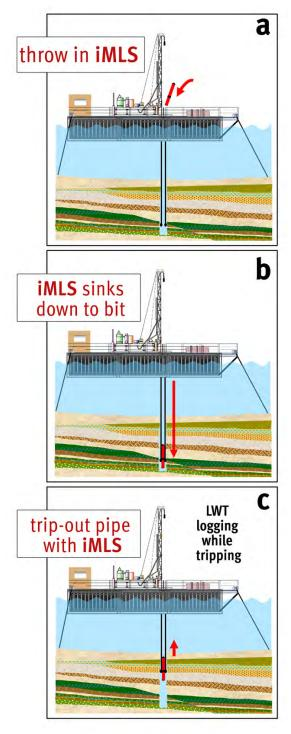
Fig. 4.6.3: Principle of Logging While Tripping (LWT) with ICDP memory logging sondes (iMLS).
