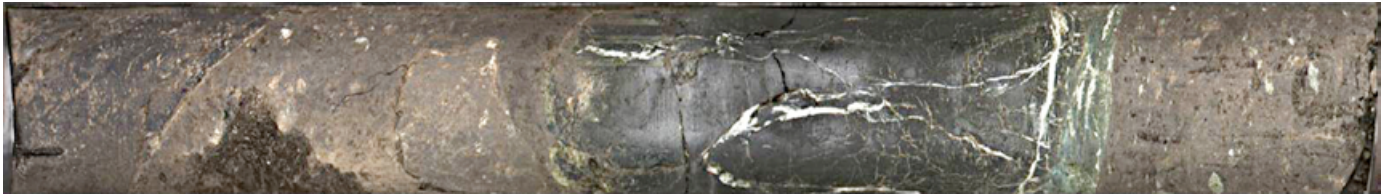
Serpentine and foliated gouge in drill core from the San Andreas Fault in California. This core was the first ever retrieved from an active earthquake fault at depth.
