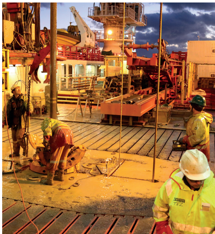
Drillers at work on the drill floor of the Fugro Synergy, a purpose-designed geo-technical vessel equipped with a permanent drilling rig (P. Robert, ECORD/IODP)
