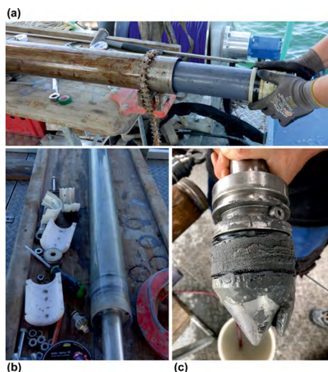
Figure 5. Opening of the coring barrel showing a 1.85 m long, sediment-filled plastic liner (gray) and core catcher (white) (a). The piston in the core-filled upper end of the liner (b). The piston after core retrieval, with sandy sediment from Lake Constance (c).
