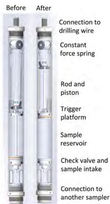
Figure 1. Cross section of a single module of the MTFS highlighting its primary components before the sampler is triggered and after.
