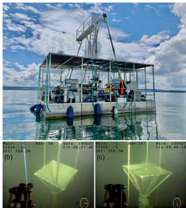
Figure 2. Hipercorig on Lake Constance during coring operations in 2019 (a). Video stills from research vessel (R/V) Kormoran remotely operated vehicle (ROV) showing the entry of coring assembly in the upper reentry cone (b). The reentry cone with hydraulic hose (green) after the coring assembly was lowered into the hole (c).
