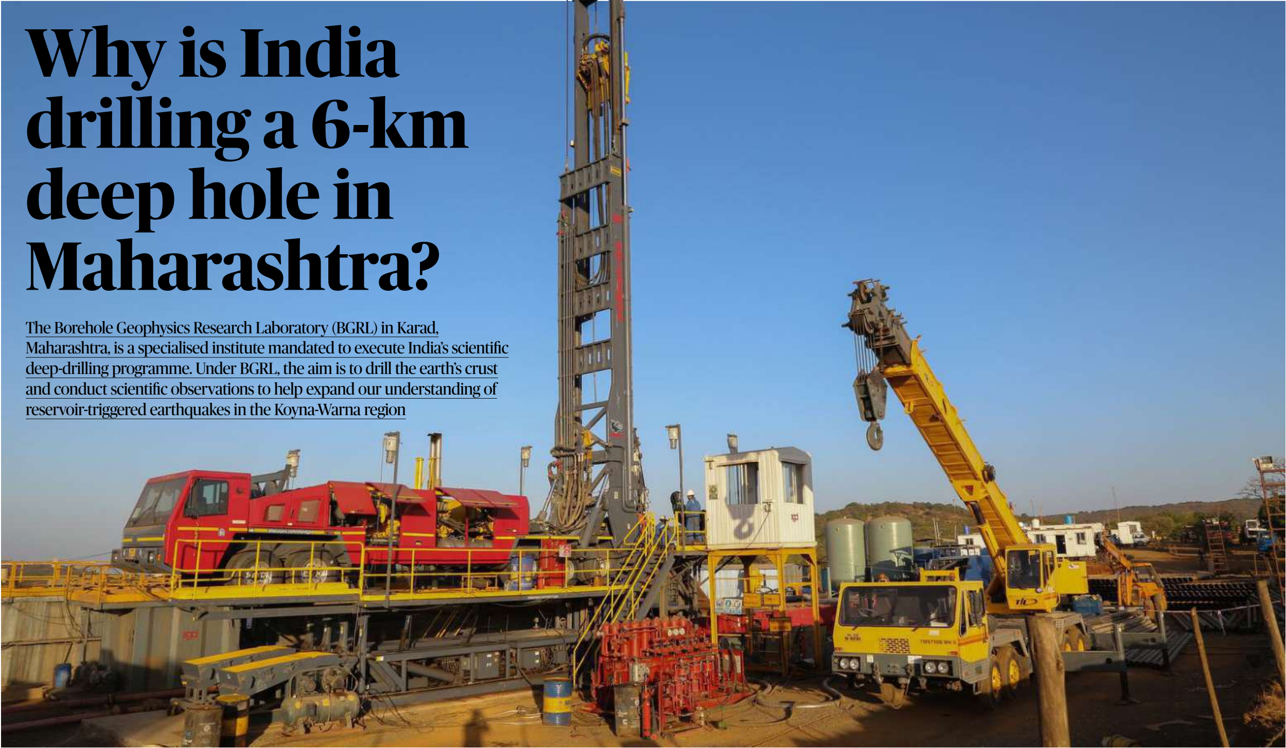
DEEP DIVE: At the deep drilling site in Koyna region, Maharashtra, the towering drilling rig is seen surrounded by associated equipment, an onsite mud logging unit, gas analysis lab, and a geological studies lab. MOES-BGRL
