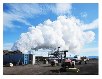
**Figure 3.** The flow of the IDDP-01 into a rock muffler produced dry superheated steam with only 0.1–0.2% of non-condensable gases. Initially corrosion products gave the steam a dark color, but after a few minutes it became clear and transparent. The condensate had a pH of 2.5–3 due to its HCL content. However, experiments on wet scrubbing to remove acid gases from the dry steam were very successful (Hauksson et al., 2014) (photograph courtesy of Kristján Einarsson).
