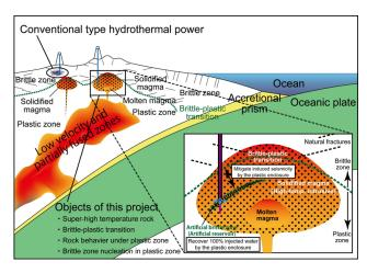
**Figure 5.** The principles behind the Japan Beyond the Brittle Project (JBBP). Figure courtesy of H. Asanuma (National Institute of Advanced Industrial Science and Technology, AIST), Japan.
