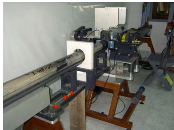
Fig. 5.9: Multisensor core logger in field lab
