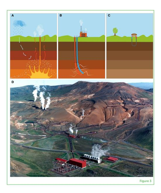
Super deep wells (several kilometers) are needed, and they work similar to deep geothermal wells but at much higher pressures and temperatures. These super deep wells can create much more energy and are thus much more effective for producing electricity.
