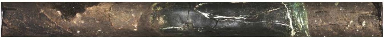
Serpentine and foliated fault gouge in SAFOD-III drill core extracted at 3194 m depth. Source: Earthscope
