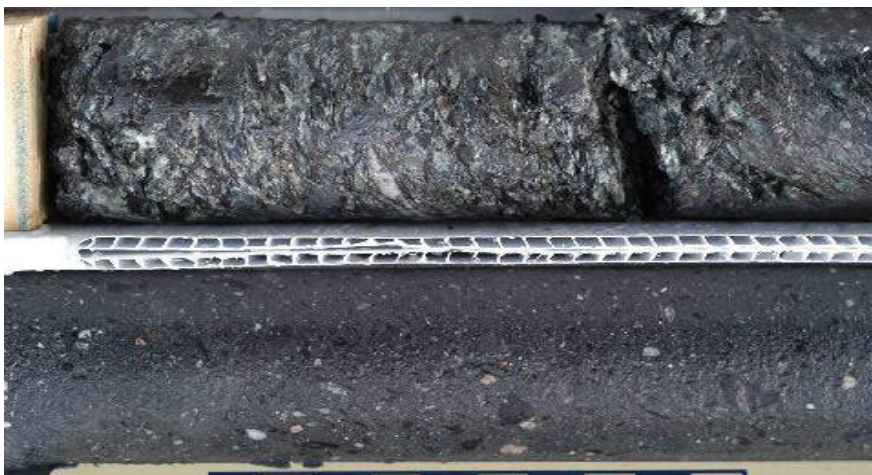
Variably brecciated schist (top) and lithic breccia (bottom) from a depth of about 1,606 m.
