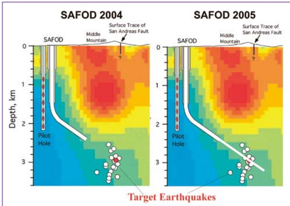
Testing Fundamental Theories of Earthquakes and Faulting: The San Andreas Fault Observatory at Depth (SAFOD) in Parkfield, Calif., U.S.A. moves into Phase 2 with directional drilling into the fault zone. During the summer of 2005 the borehole is expected to pass through the entire fault zone (<http://safod.icdp-online.org>).
