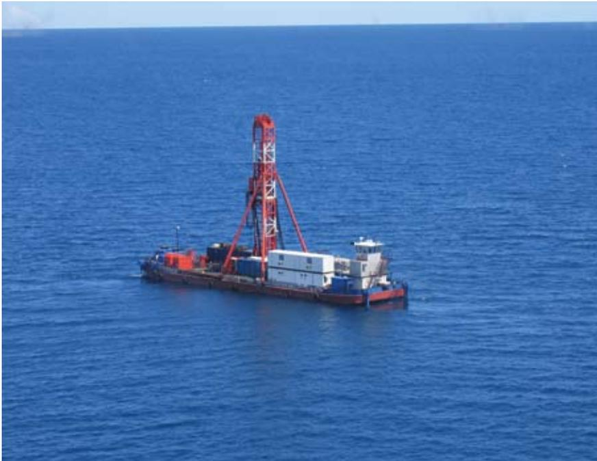
ICDP began NSF funded lake drilling operations on Lake Malawi, Africa, in March 2005. A modified local barge with mounted heave-compensated drill rig and four 360° outboard thrusters for station-keeping was used to drill up to 380 m sediment core with >95% core recovery in almost 600 m water depth (<http://www.icdp-online.org>).
