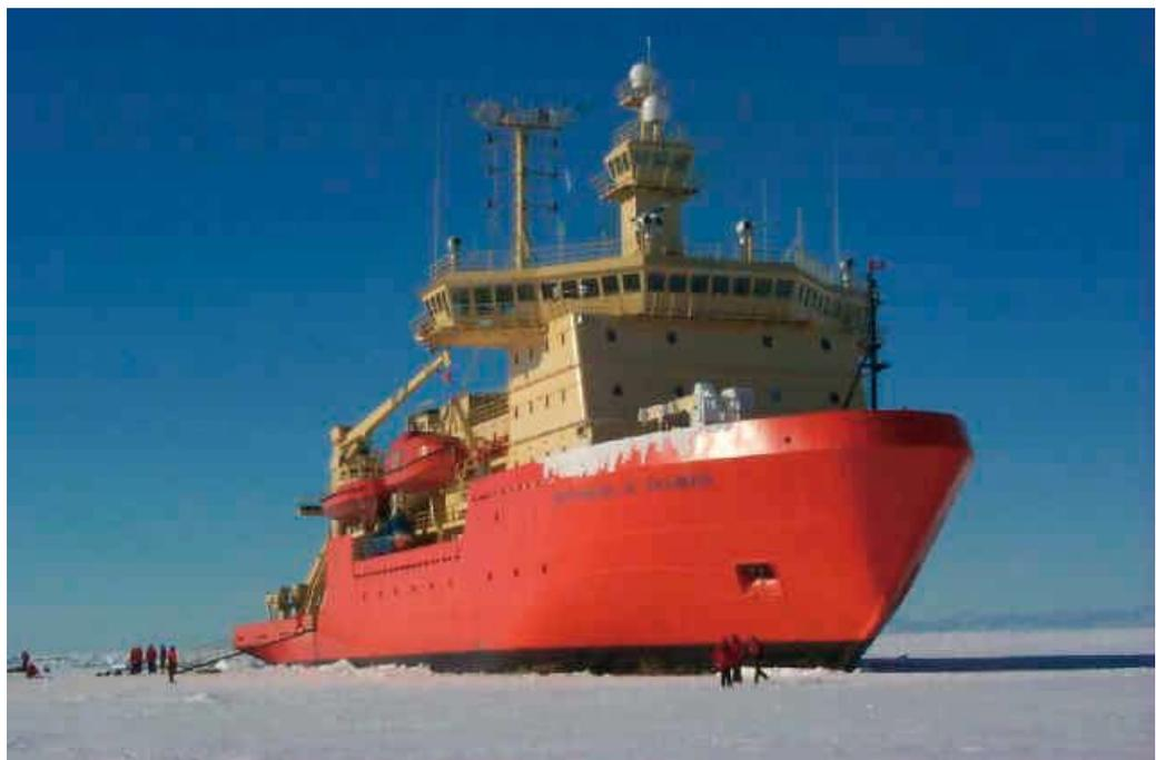
The process of planning to install the R-50 rig onto the *Palmer* brought with it many unexpected problems. The major hurdle was that the rig adds so much mass at heights above deck that the vessel would not meet damage-stability criteria defined by the U.S. Coast Guard. After analyses by several naval architects and tests performed on the ship, additional ballast was installed to allow the R-50 rig to be safely mounted on board.
