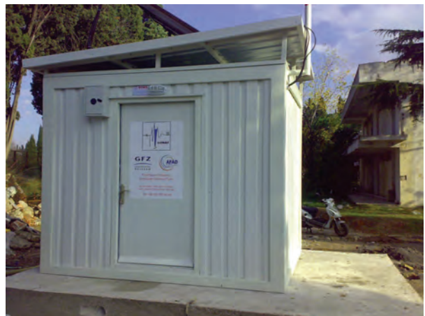
Fig. 7.6: Recording container on top of the monitoring wellhead Tuzla-1 (courtesy: GONAF)
