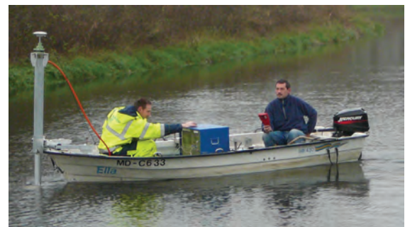
Fig. 3: Shallow water survey with parametric sub-bottom profiler SES-2000 consisting of a transducer and a control unit and consuming less than 500 W (© Innomar Technologie GmbH 2006)
