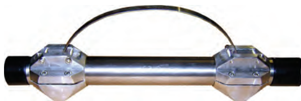
Fig. 7.4: Spring bow de-centralizer hole lock concept (photo: SAFOD project)
