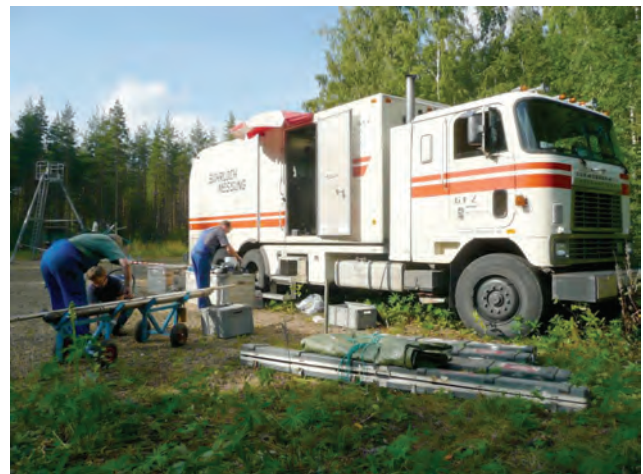
Fig. 7.1: Truck-based GFZ wireline unit
