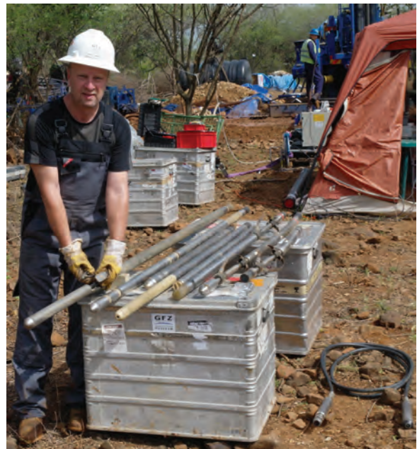
Fig. 6.3: OSG slimhole logging sondes at drillsite
