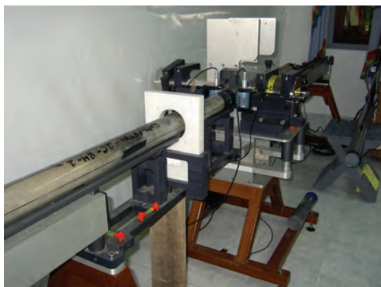
Fig. 8.1: Multi-sensor core logger in field lab
