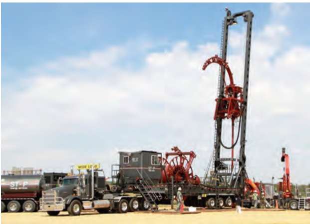
Fig. 7.3: Coiled tubing operation from a flat-bed truck with truck-mounted derrick
