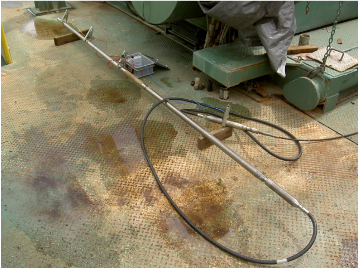
DLL on-site verification with the calibrated resistances box (bridle cable length is 6 m)
