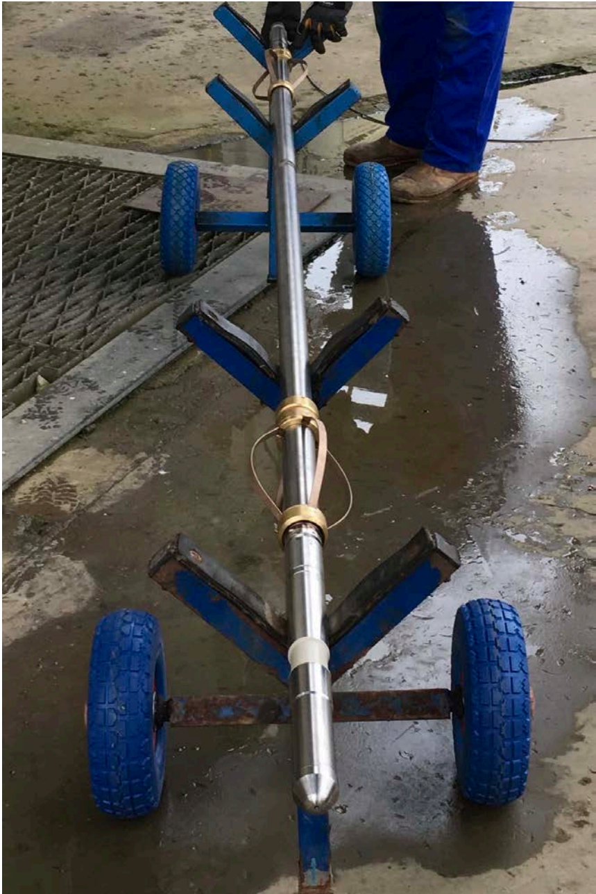
ABI43-2G - slimhole wireline Acoustic Borehole Imager tool including total GR
