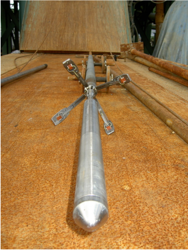
DIP - slimhole wireline Dipmeter tool
