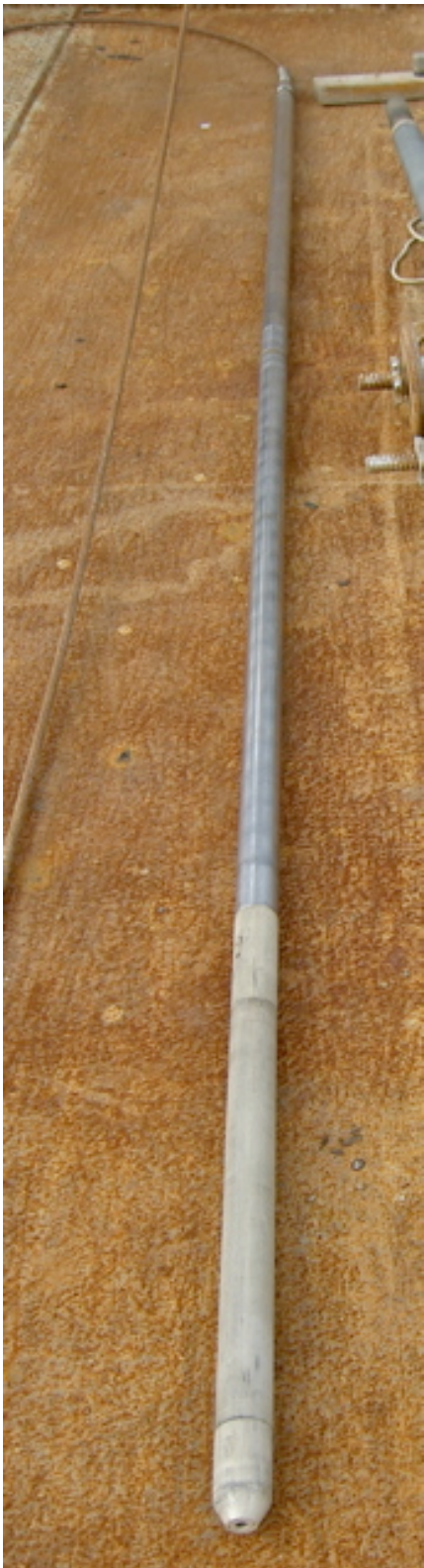
MS - slimhole wireline Magnetic Susceptibility tool (mounted below telemetry sub)
