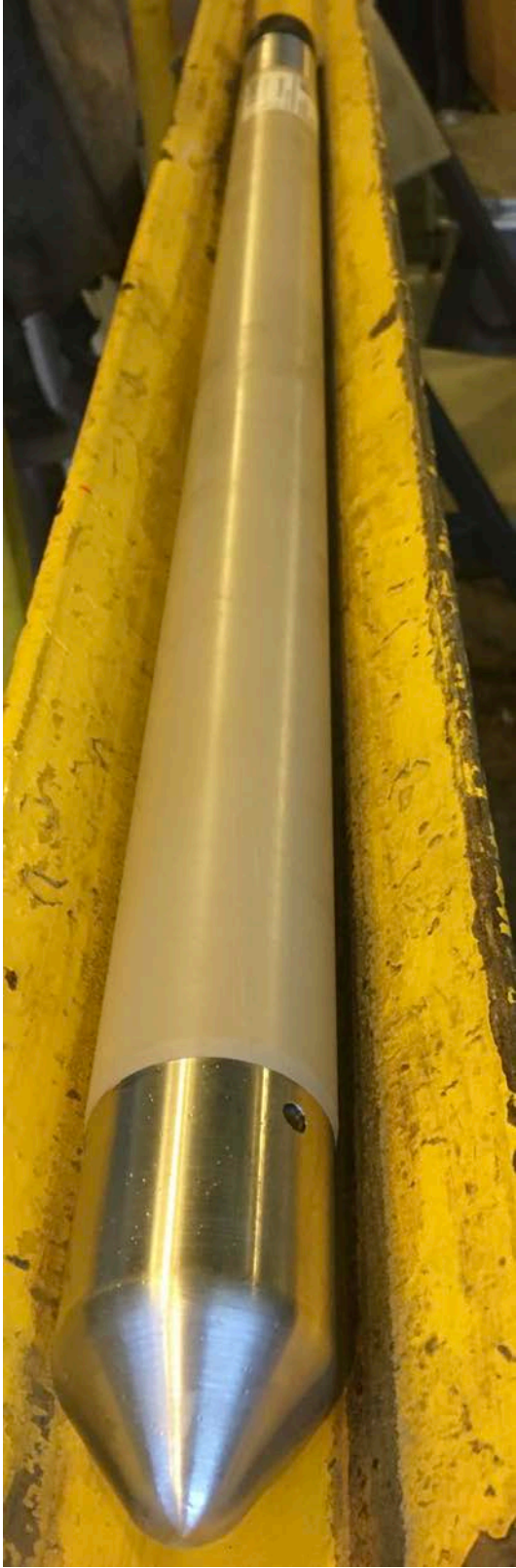
SP – slimhole wireline Spontaneous Potential (analog, standalone sonde w/o GR)
