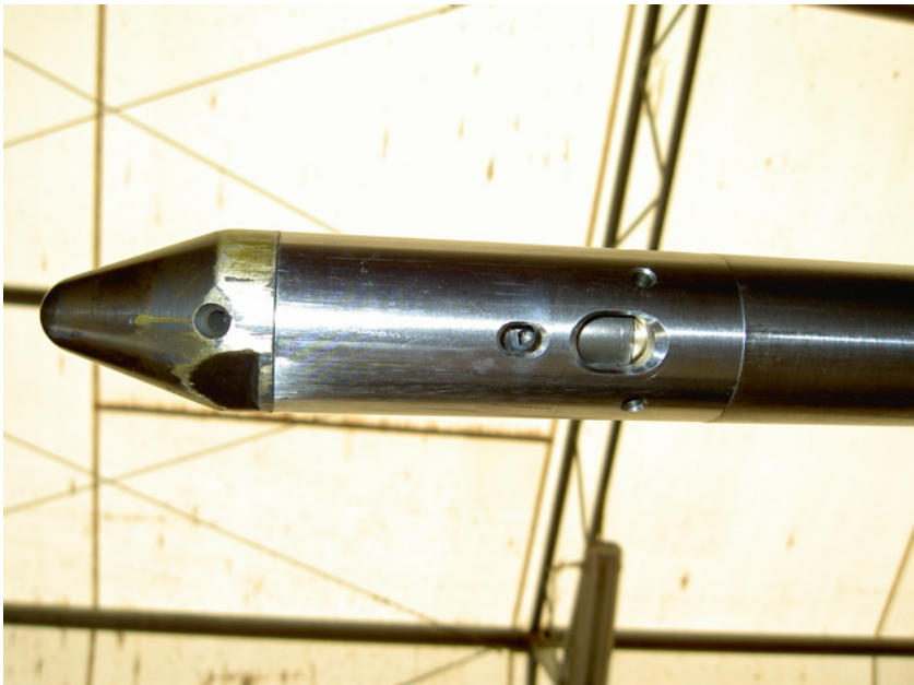
FS tool bottom with sample entrance port
