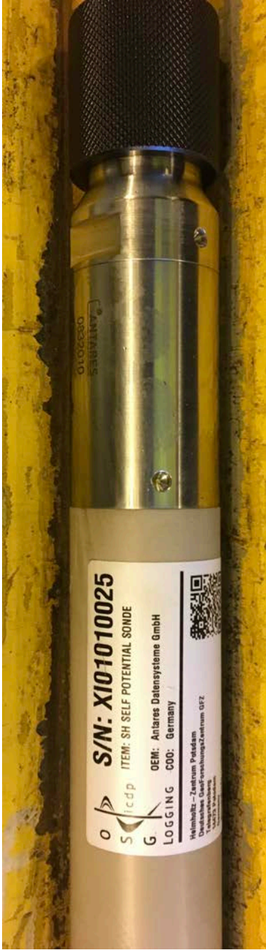
SP – slimhole wireline Spontaneous Potential (analog, standalone sonde w/o GR)
