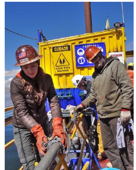
Core on deck! After core arrival, the core barrel is cleaned and the core recovery is determined.
