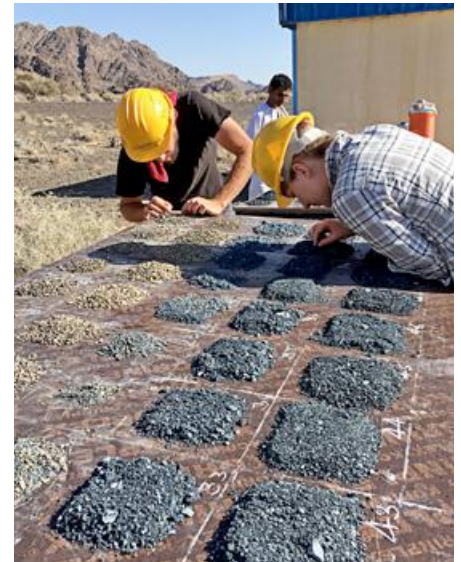
Scientists from the Oman Scientific Drilling Project are investigating rock chips (cuttings). When no drill cores are available, cuttings are the means of choice.
